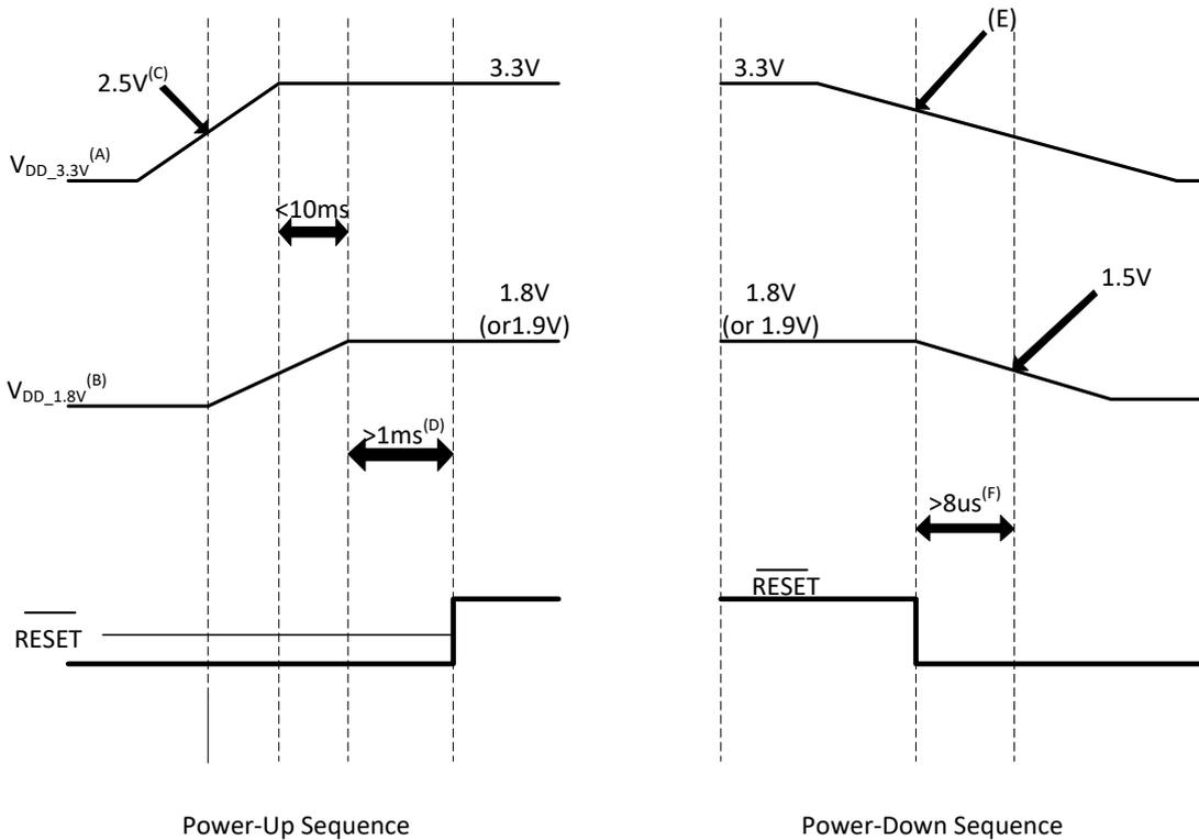
A.  $V_{DD\_3.3V}$ - $V_{DDIO}$ ,  $V_{DDAIO}$ ,  $V_{DDA1}$ ,  $V_{DDA2}$ ,  $AVDDREF$
