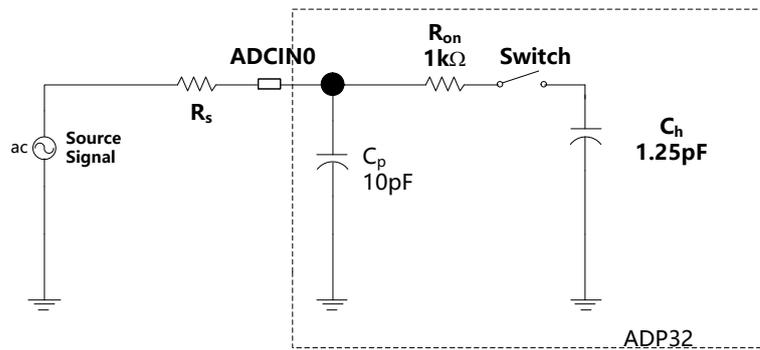
**Typical Values of the Input Circuit Components:**
